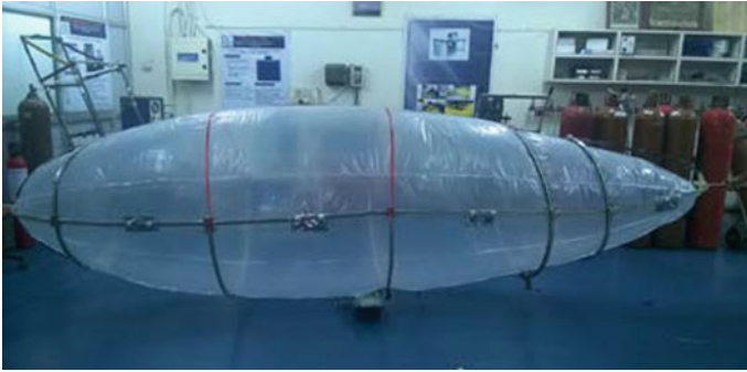
Fig. 5 Semirigid airship fabricated by Loharkar et al. [13]
